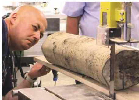
Pic.2 ...before using an MDF board to stabilise the log on the table and run against the fence to create the first flat side...
